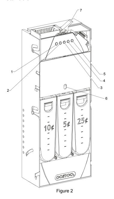
Description Description Item Item LED Indicator Mode Button 5 2 Inventory Button − Left Hopper (10¢) Hopper Release Lever 6 3 Inventory Button − Center Hopper (5¢) 7 Escrow Lever Inventory Button – Right Hopper  $(25\not\epsilon)$
