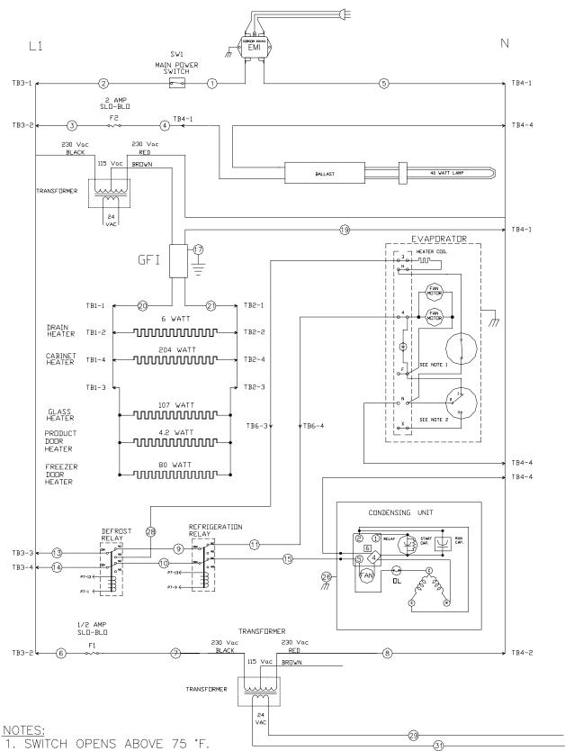
2. TERMINALS 2 & 3 SHORTED WHEN COIL IS >55 °F. TERMINALS 1 & 2 SHORTED WHEN TEMPERATURE FALLS BELOW 35 °F.
