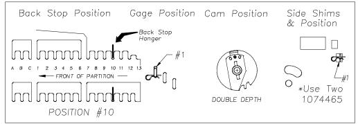
**Note:** \*Due to the variance of diameter of the product from the PET Mfg. two flat shims will be required to properly vend 20oz. Powerade. If product exceeds the dimension of 2.905 +.080 remove shims accordingly.
