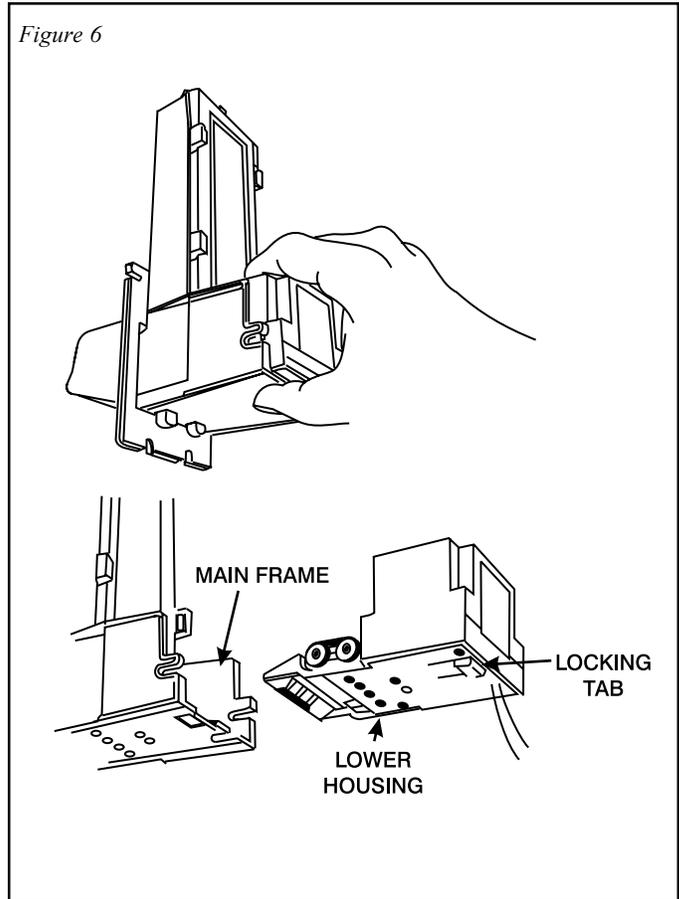
**Removing the Intermediate Frame
