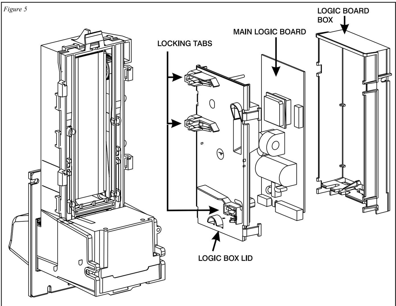
**Removing the Lower Housing
