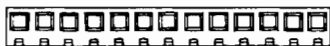
AMP IN-LINE CONNECTOR .156 CTRS. 2 PIN - 380232 7 PIN - 380232-1 18 PIN - 380232-3 13 PIN - 380232-2 16 PIN - 380232-11 19 PIN - 380232-4 4 PIN - 380232-7 3 PIN - 380232-6
